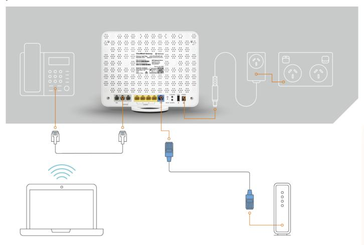
Using an ethernet network cable, connect your modem from its WAN port to the blue WAN port on your NetComm modem. We generally activate the next available Uni-D port – starting with Uni-D 1. We will detail your Uni-D port number in our emails to you.
