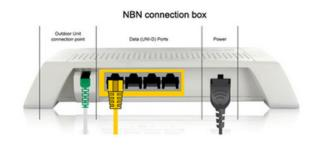
Using an Ethernet network cable, connect your Wi-Fi router from its WAN port to the relevant Uni-D port on the nbn® Connection box. We generally activate the next available Uni-D port – starting with Uni-D 1. We detail your Uni-D port number in our emails to you.
